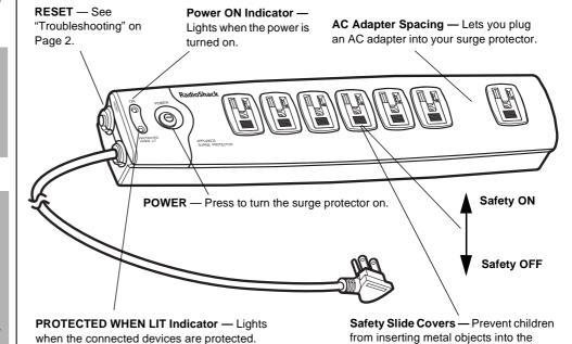
**Power Shutdown Protection** — Protects the connected appliances from being damaged by shutting down power when surge protection is depleted (see "Troubleshooting" on Page 2).
